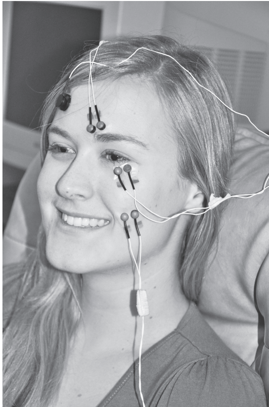
Figure 3.1 Electrodes placed over the zygomaticus major (cheek), corrugator supercillii (brow), and orbicularis oculi (eyeblink) regions. The electrode on the right forehead is being used as a ground (Photo: Eric Vanman)
